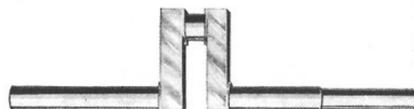
D—Crank Shaft. The crank shaft of our engines is made of one solid piece of steel without weld or shrink, and is milled to shape from a single piece of steel twice its finished size.
