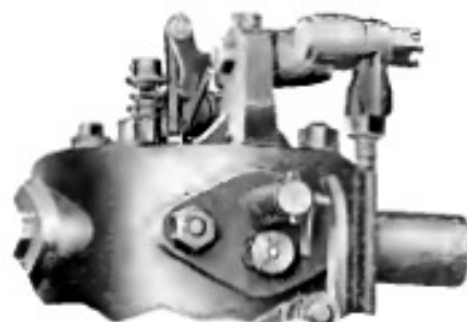
Cylinder Head Showing Ignition Trip and Valve Gear
