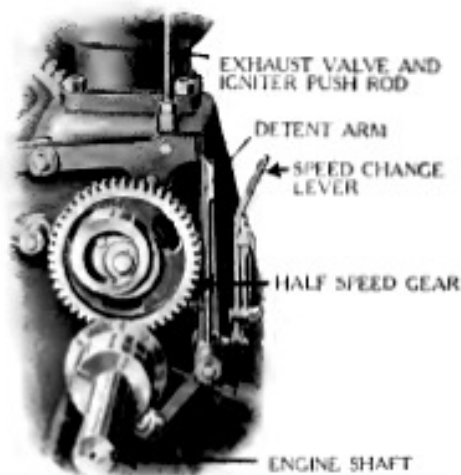
Speed-Changing Device and Governor (Flywheel Removed)
