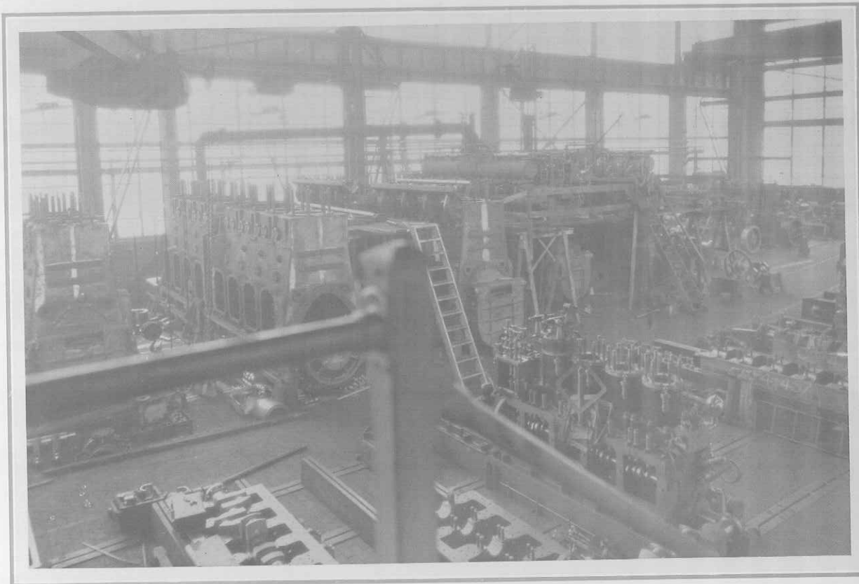
A corner of the diesel erecting plant, showing a group of Bessemers in the process of being assembled.
