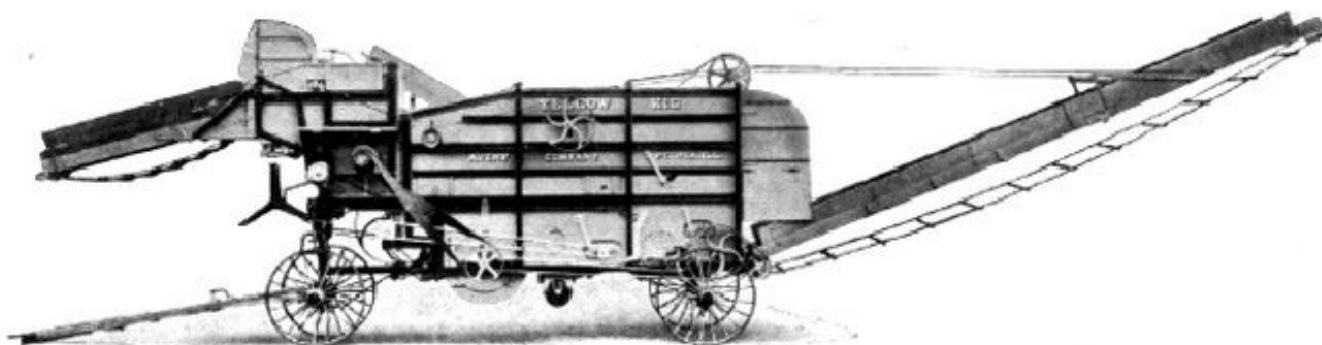
Right Hand Side of an Avery "Yellow Kid" Thresher Fitted with Self-Feeder and Common Stacker
