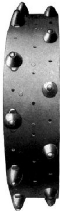
HEART SHAPED SPUDS. In this illustration the rear wheels are equipped entirely with Heart Shaped Spuds, which can be furnished if desired.
