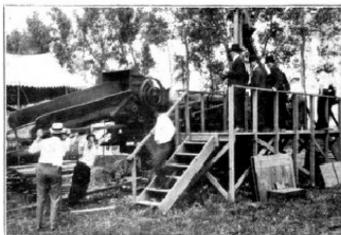
Threshing a 2 x 12-inch Oak Plank at the Fair to Show the Strength of Avery Jumbo Tool Steel Teeth.
