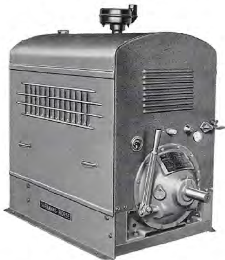
The Power Take-Off end of the FM-65 Electric Start Power Unit. The rear panel shows the oil pressure gauge, starting switch, ignition switch and key, ammeter and governor adjusting screw.
