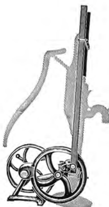
KJ Clutch Jack With Complete En- circling Gear Guards
