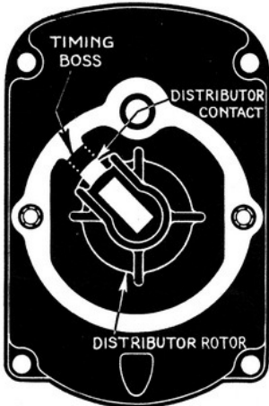
Fig. 3 - Timing Diagram should be made to the engine instruction book for details concerning the timing marks of the particular engine. Turn the engine over until the timing marks coincide, indicating that it is in advance spark position (#1 cylinder).
